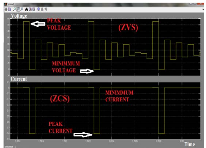
Fig 11:- Switching characteristics of main switch M a .
